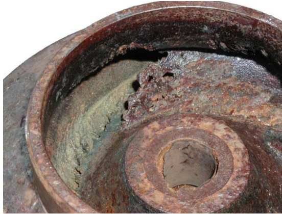
Figure 1. Suction side Cavitation
