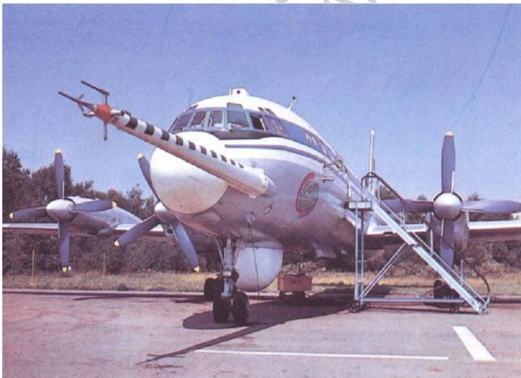
Figure 1: Flying laboratory “Ilyushin-18” equipped with different sensors for measurements of atmospheric parameters and tools for cloud seeding. It was used in various research and operational projects for weather modification
