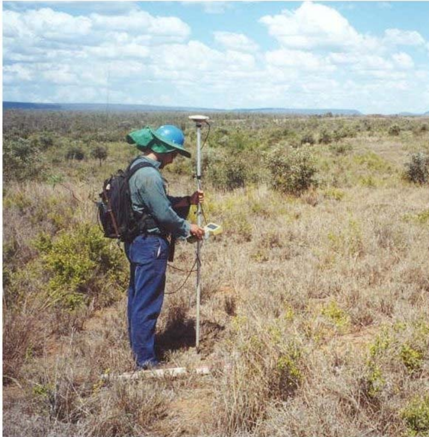
Figure 1: Gathering ground magnetic data as part of a coal exploration program
