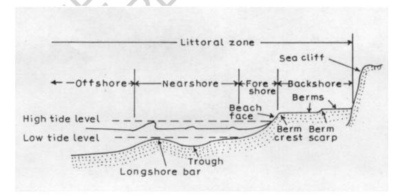
Figure 1. Terminologies used to describe beach and nearshore profiles
