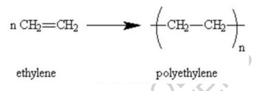
Scheme 1. Polymerisation of ethylene
