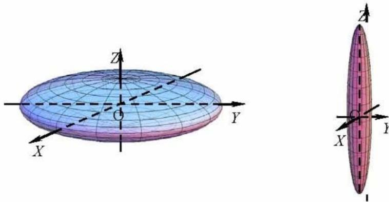
Figure 2. Strongly oblated and strongly prolated ellipsoidal QDs.
