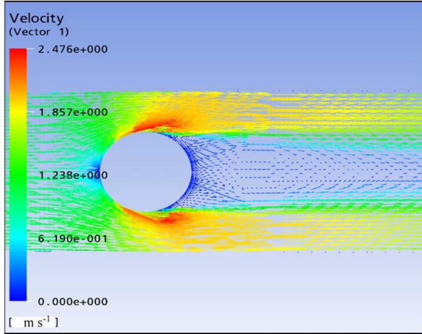
Figure 1(b). A stationary flexible cylindrical tube in an externally cross flowing fluid: Typical instantaneous flow field around the cylinder subjected to cross-flow in a rectangular duct
