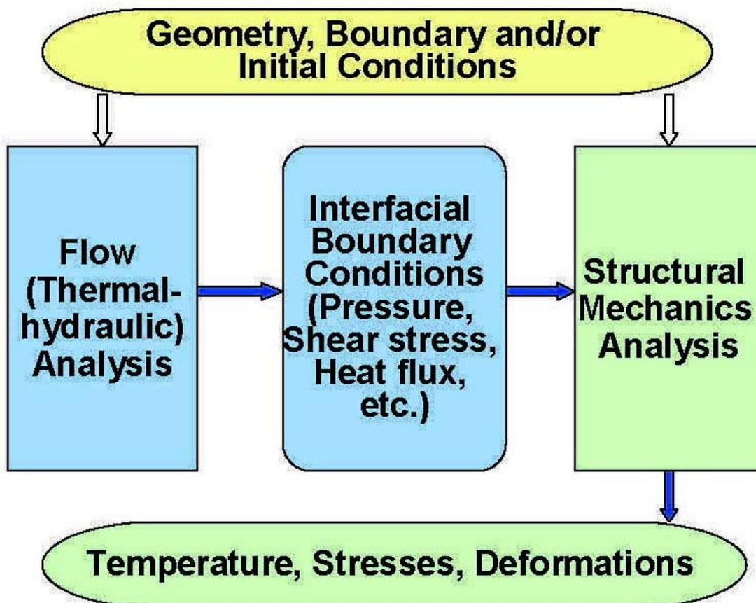
Figure 2. One-way separate analysis method
