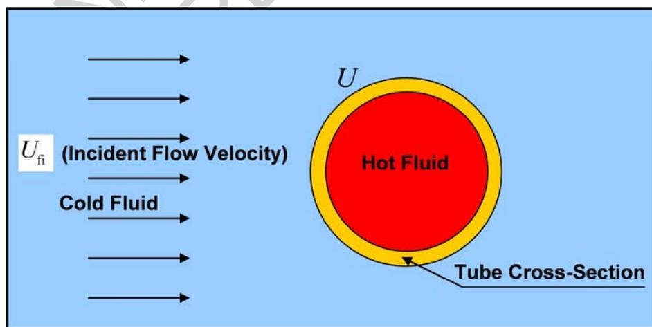
Figure 1(a). A stationary flexible cylindrical tube in an externally cross flowing fluid:
