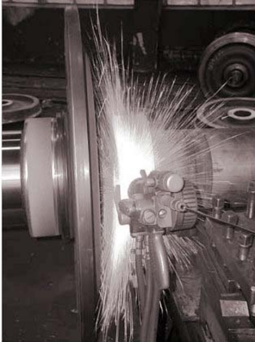
Figure 8. Photography of wire flame spraying
