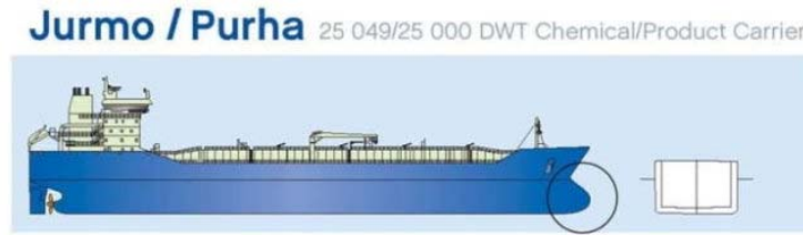
Figure 13. A ship having an ice bulb, circled in the figure ( www.nesteoil.com ).
