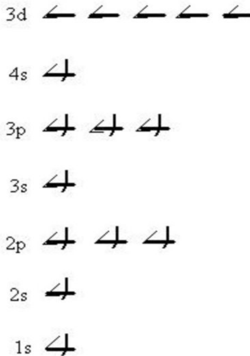
Figure 1. Energy Level Diagram for a Manganese Atom Showing the Electron Occupation.
