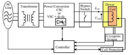
Figure 1: Components of a Typical SMES System
