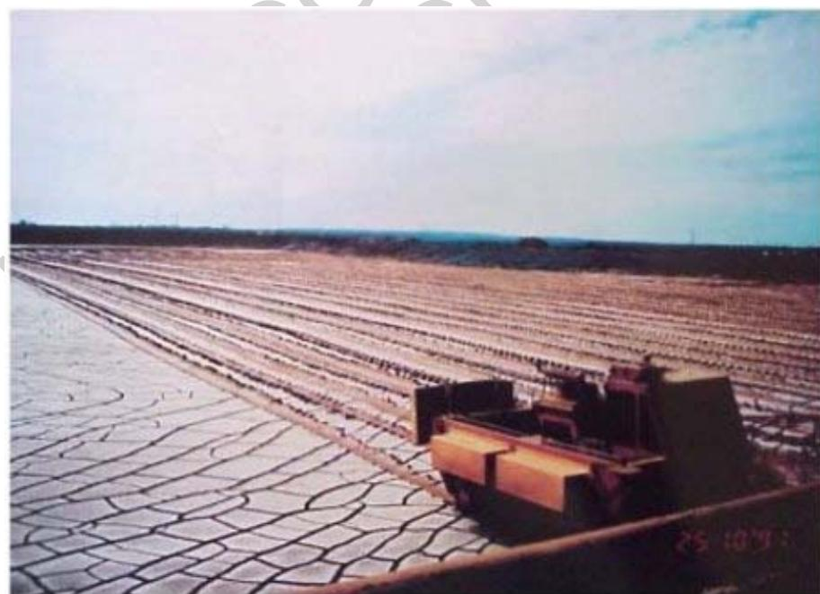
Figure 7. Alcoa Western Australia, bauxite waste dry stacking
