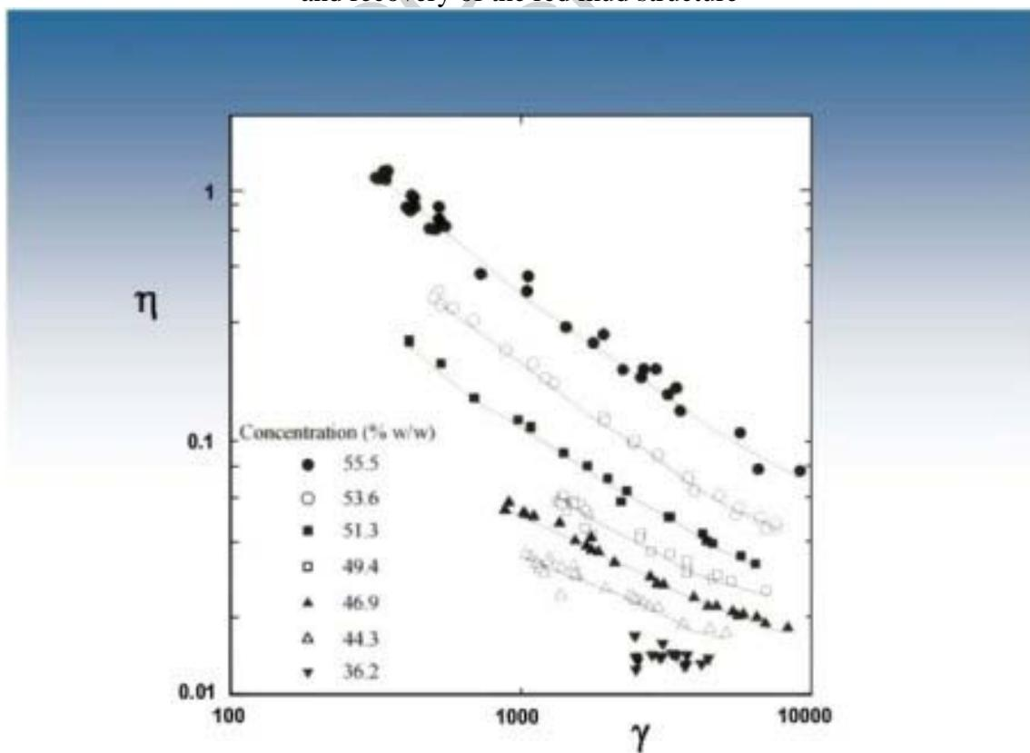
Figure 5. Red mud equilibrium viscosity shear rate data
