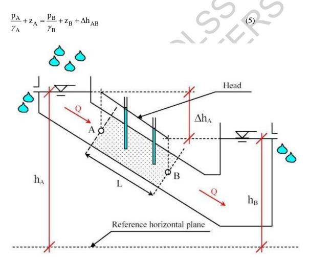
Figure 3. Hydraulic system in a porous medium with fluid motion from A to B (from higher to lower head levels).
