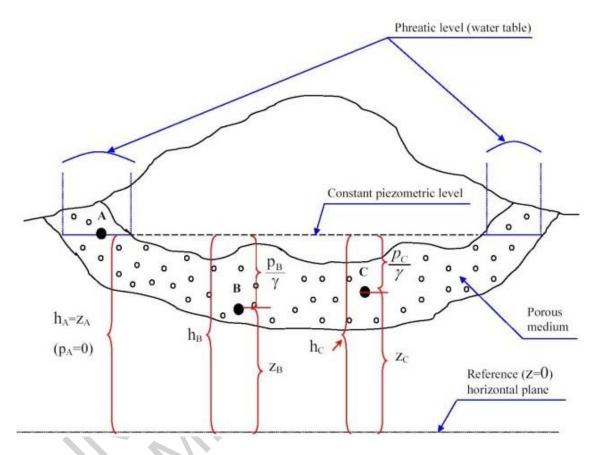
Figure 2. Aquifer under no flow conditions (static system). Observe that points A, B and C have the same head level, but a different pressure. Point A has atmospheric pressure (taken as 0).
