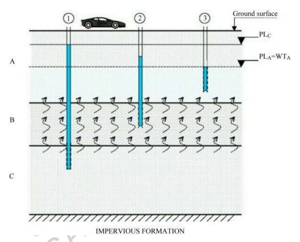
Figure 1. Classification of aquifers in terms of hydrostatic pressure (no pumping conditions)
