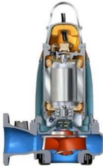
Figure 1: Submersible sewage pump. Liquid enters from the bottom and is discharged through the expander at left. Courtesy of ITT Flygt Corp., Trumbull, CT, USA
