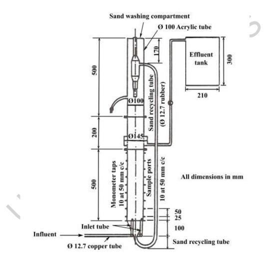
Figure 3. Sectional view of mobile bed filter
