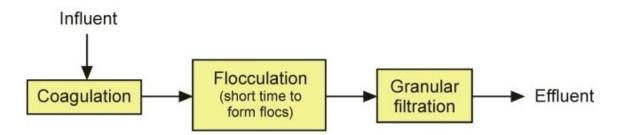
Figure 1. Process flow scheme of direct filtration
