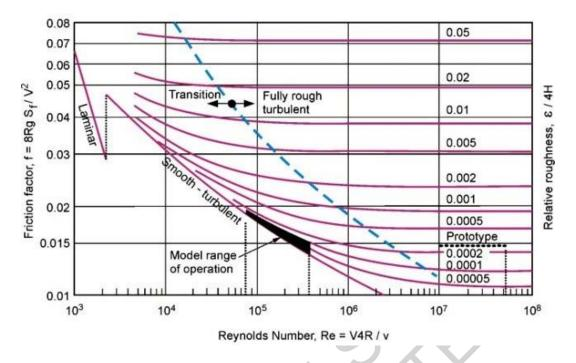
Figure 1. Process function diagram for friction, showing the relationship between friction factor and Reynolds number
