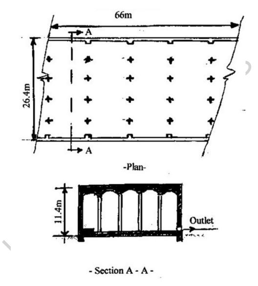
Figure 2(a). A Roman reservoir with vaulted roof supported by columns
