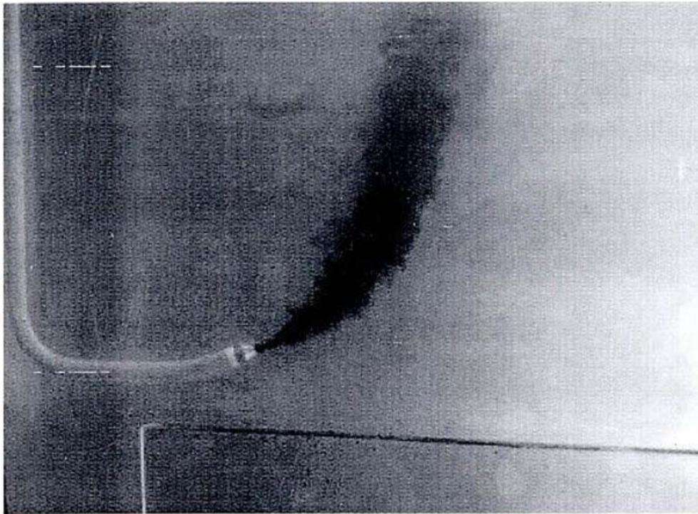
Model of the Wah Fu Outfall, Hong Kong. This shows a single round, buoyant jet in still water. ( $F_o = 6.3$ , discharge angle =  $20^\circ$ )
