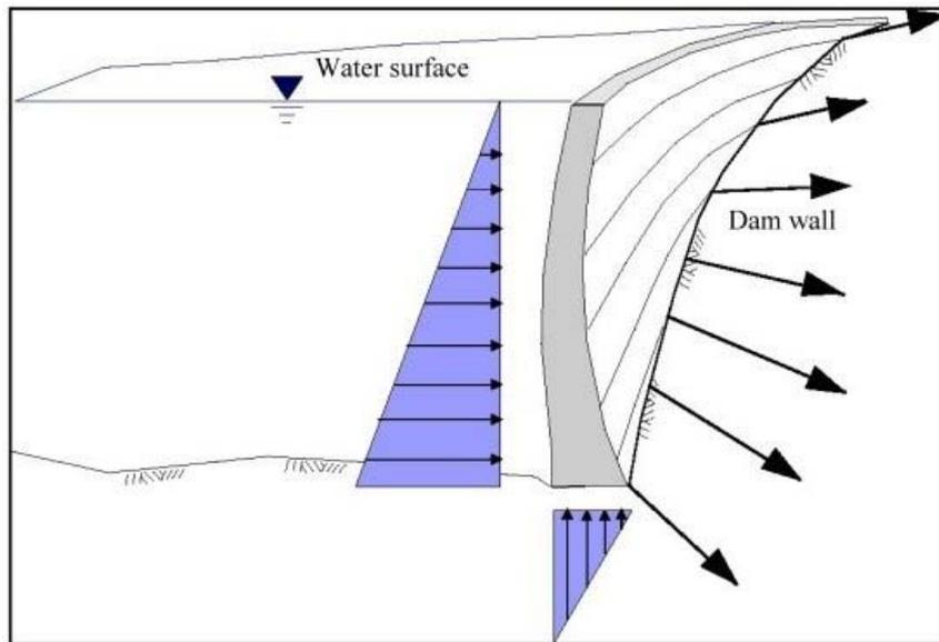
Figure 3. Hydrostatic loads
