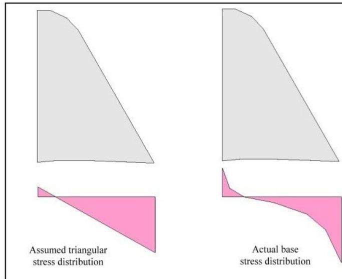
Figure 8. Uplift distribution in a gravity dam
