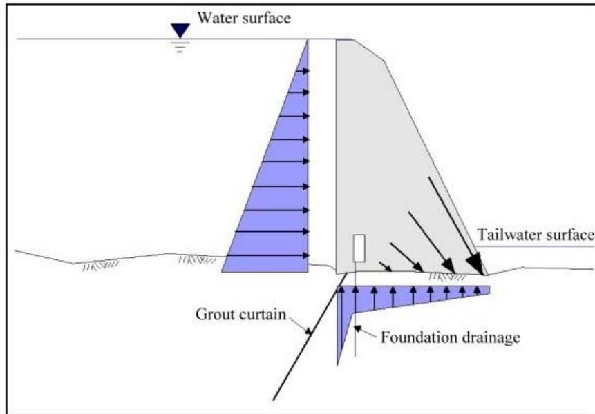
Figure 7. Loads and forces in a gravity dam
