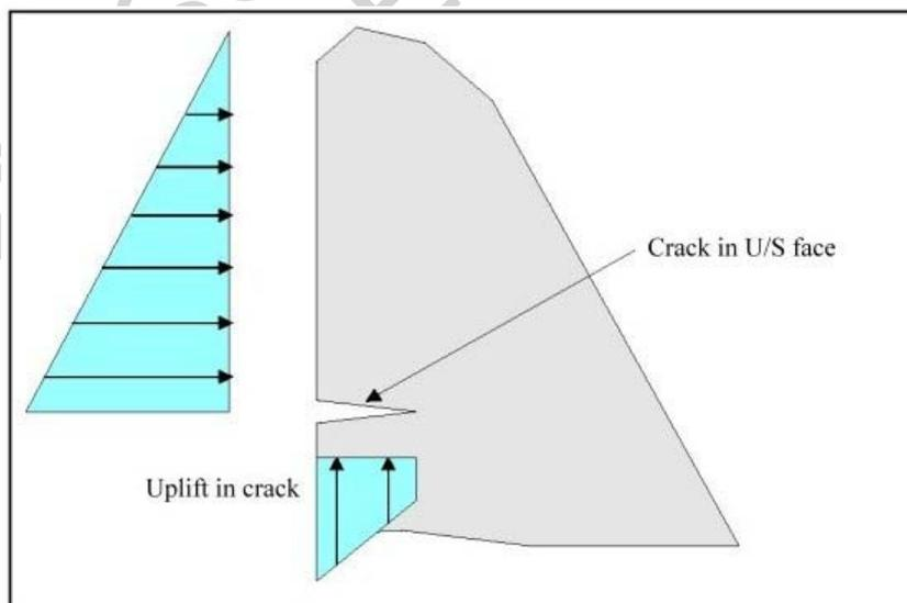
Figure 9. Uplift in cracked section in a gravity dam
