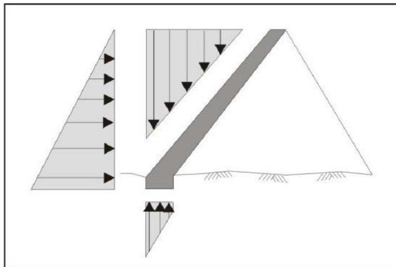
Figure 10. Forces on a buttress dam
