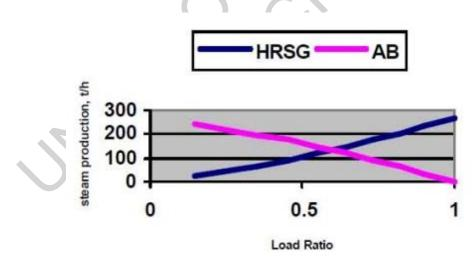
Figure 7 HRSG and AB steam productions at various GT load ratios
