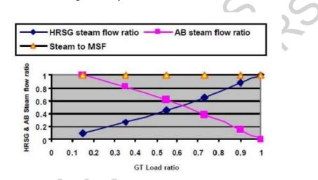
Figure 2 HRSG and AB steam flow ratios for various GT load ratios
