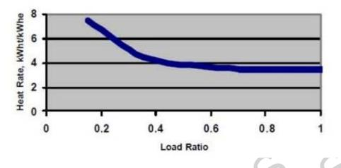
Figure 6 Heat rate versus load ratio for GT model 9171E gas turbine (ambient Temperature =  $20^{\circ}$ C)
