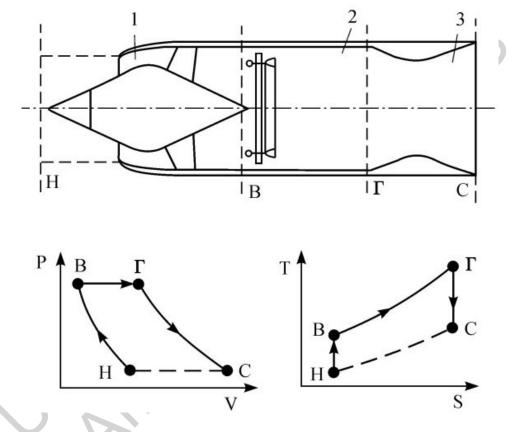
Figure 3: Diagram of the scramjet and its cycle in coordinates *p*-*V* and *T*-*S*.
