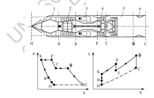
Figure 2: Diagram of the turbojet with after burner and its thermodynamic cycle in coordinates p-V
