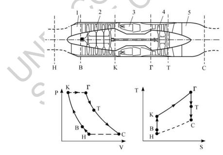
Figure1: Diagram of the turbojet and its thermodynamic cycle plotted in coordinates p-V and T-S. The dots show parameters in the cardinal cross section of the engine
