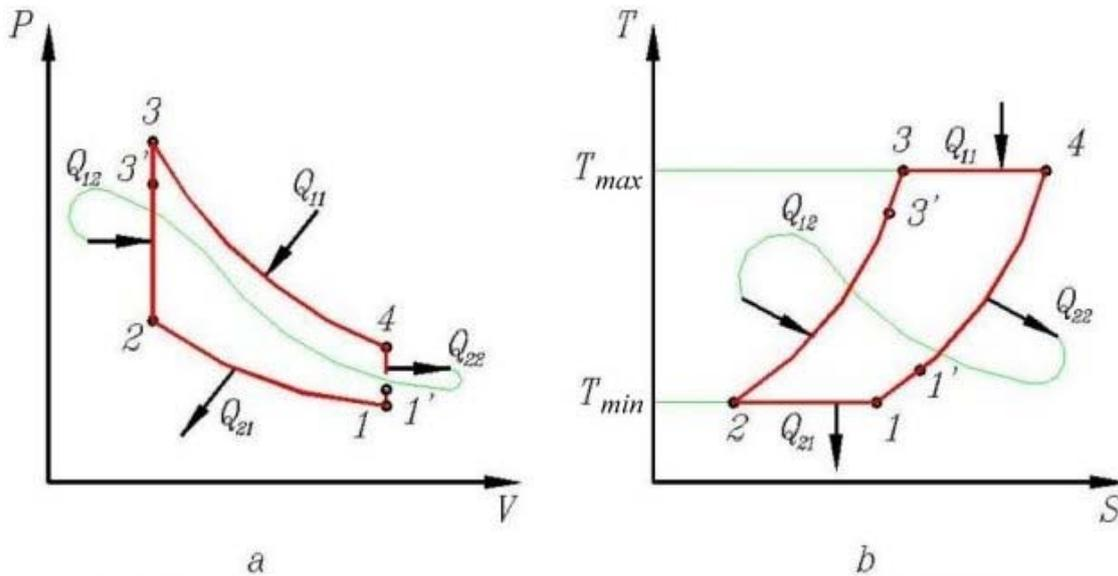
Figure 1. Thermodynamic cycle of Stirling engine
