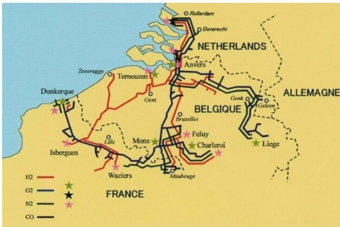
Figure 1. Hydrogen Pipeline Net Work in Northern France - Belgium
