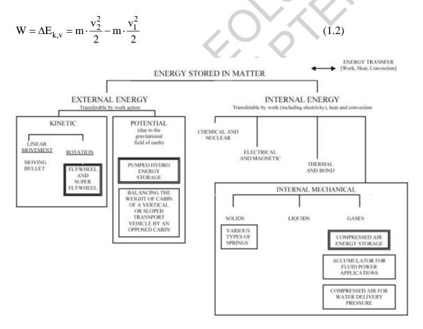
Figure 1: Three Main Types of Mechanical Energy Storage: Kinetic Potential and Internal Mechanical
