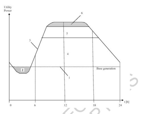
Figure 3: Approximate Variation of Utility Power Demand and Satisfying it by Various Power Sources: i) Base load power plants together (nuclear, hydraulic, wind), ii)Surplus electrical power absorbed by utility energy storage plants, iii) Demand variation of utility grid, iv) Gas turbines and other smaller power plants, v) Power produced by cogeneration and independent private power plants, vi) Power delivered by utility energy storage plants
