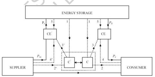
Figure 2: Control of Energy Flow to and from a Mechanical Energy Storage System CE, CE': Conversion Equipment; C, C': Control System; Full lines indicate flow of energy or energy carrier and dashed lines indicate signal transfer
