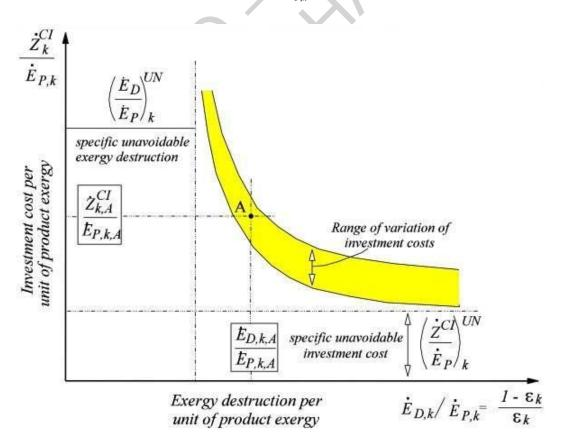
Figure 1: Expected relationship between investment cost and exergy destruction (or exergetic efficiency) for the *k*-th component of an energy conversion system.
