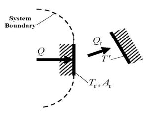
Figure 4. Radiated heat
