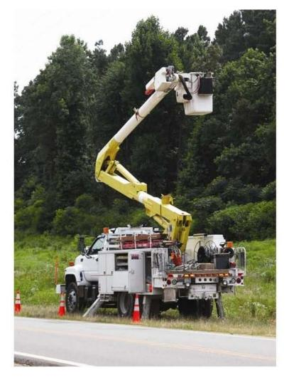
Figure 2. Mobile Elevated Working Platform © NEBOSH
