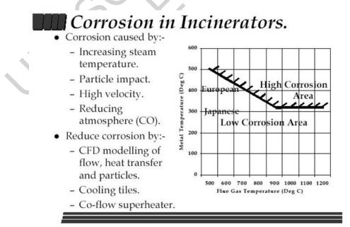
Figure 1. Corrosion in incinerators
