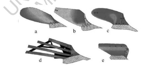
Figure 4.Various shapes of moldboard: a) general-purpose; b) digger; c) semi-digger; d) slatted; e) diamond (Peruzzi A. and Sartori L. 1997).
