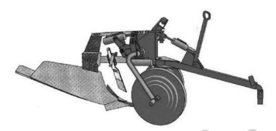
Figure 5. Trailed single-furrow deep-digger plow with hydraulic controls (Peruzzi A. and Sartori L. 1997).
