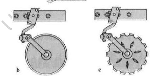
Figure 2. Type of coulters: a) shin coulter (incorporated in the front part of the moldboard); b) plain-edge disk coulter; c), ripple-edge disk coulter (Peruzzi A. and Sartori L. 1997).
