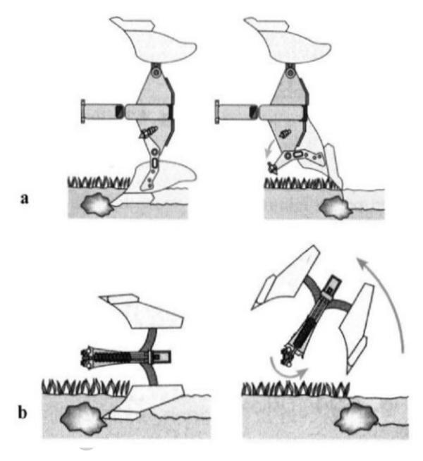
Figure 7. Examples of overload protection devices: a) breaking bolt; b) spring-trip or hydraulic reset (Peruzzi A. and Sartori L. 1997).
