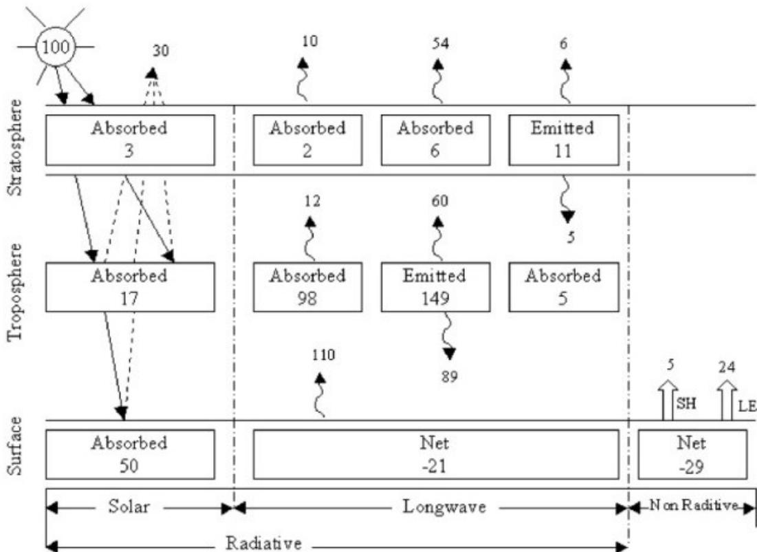
Figure 2. Radiative and nonradiative energy flow diagram for Earth and its atmosphere
