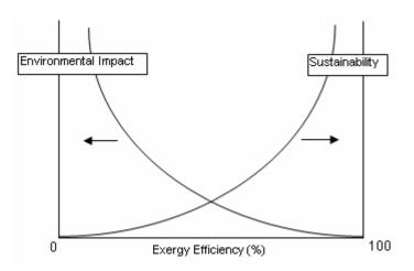
Figure 5. Qualitative illustration of the relation between the environmental impact and sustainability of a process, and its exergy efficiency.
