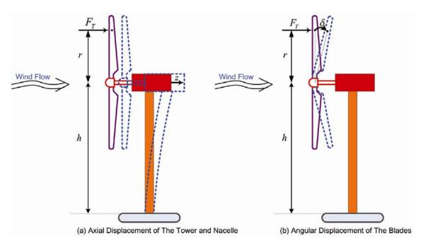
Figure 7. Structural dynamics of HAWTs
