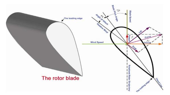
Figure 5. Aerodynamic principle of HAWTs
