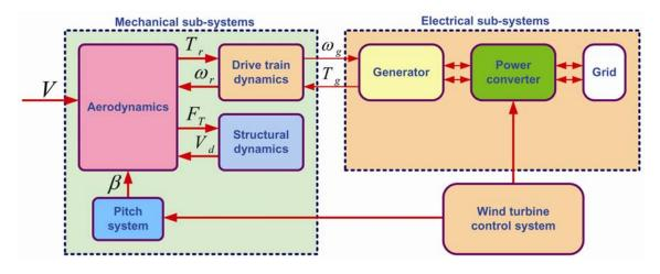
Figure 4. Wind turbine subsystem block diagram
