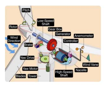
Figure 2. Basic components of a HAWT (Courtesy of the U.S. Department of Energy: http://www1.eere.energy.gov/wind/wind\_how.html)
