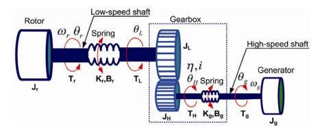
Figure 8. Flexible drive train of HAWTs
