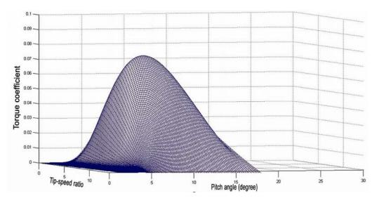
Figure 6. Torque coefficient is a function of the tip-speed ratio and pitch angle
