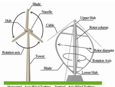
Horizontal - Axis Wind Turbine Vertical - Axis Wind Turbine
