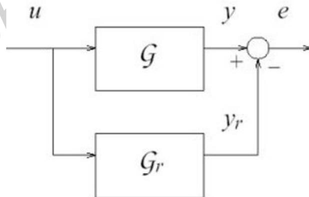
Figure 1: Single Component Model Reduction
