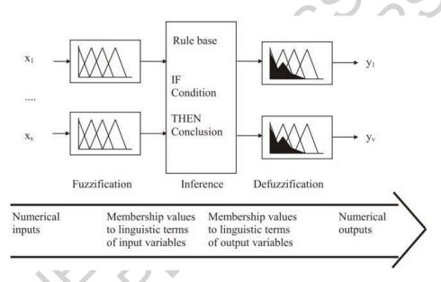
Figure 2: Structure of a fuzzy system with numerical inputs  $x_1, ..., x_s$  and numerical outputs  $y_1, ..., y_v$
