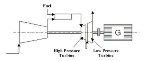
Figure 2: Two shaft, single cycle power block.
