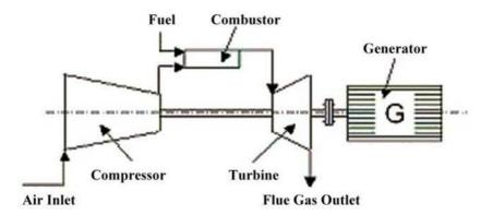
Figure1: Single shaft power block.
