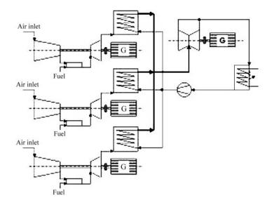
Figure 5: Multi shaft, combined cycle power plant setup.
