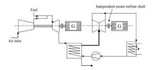
Figure 4: Double shaft, combined cycle power plant with separate generators for gas turbine and steam turbine.
