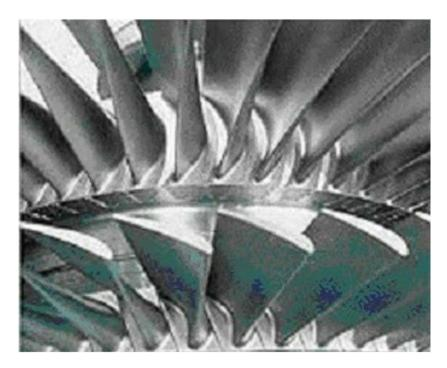
Figure 6: Compressor blades of a heavy-duty gas turbine.
