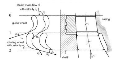
Figure 6. Guide wheel and rotating wheel. c<sub>i</sub>: absolute velocities; w<sub>i</sub>: velocities relative to the rotating wheel
