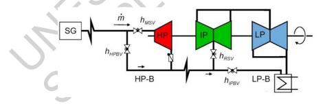
Figure 9. Turbine with HP and IP bypass station
