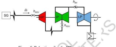
Figure 8. Reheating after the HP section
