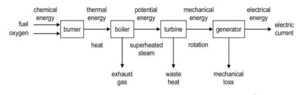
Figure 2. Energy conversion in a fossil-fuelled power plant
