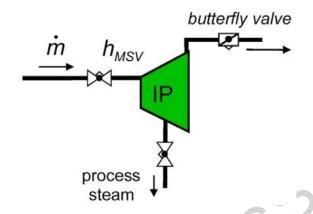
Figure 10. Process steam extraction, part drawing
