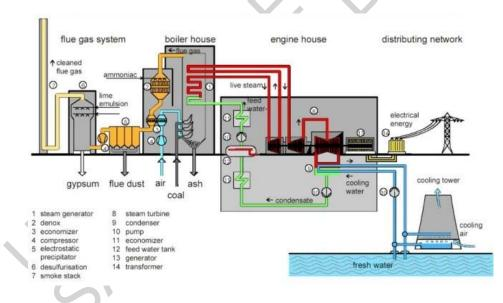
Figure 3. Components of a fossil-fuelled steam power plant; schematic overview
