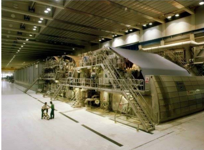
Figure 3. Typical modern paper machine (Courtesy Metso Paper, Inc).
