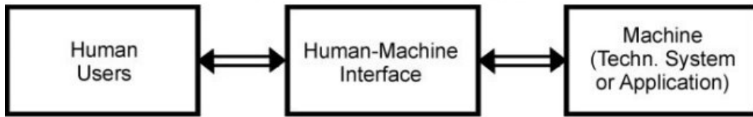
Figure 1: The whole human-machine system (HMS) with human users, human-machine interface, and the machine.
