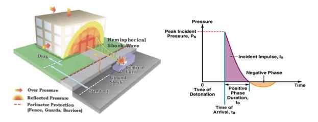
Figure 1. Schematic view of air-blast pressures acting on a building and pressure-time history of loading
