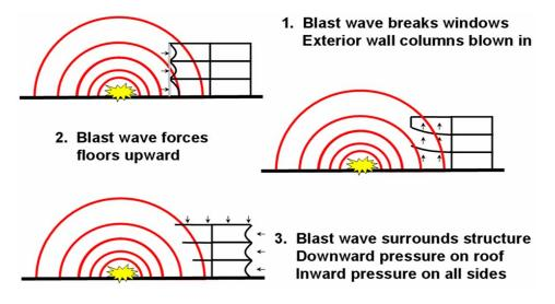
Figure 2. Damage pattern due to explosion
