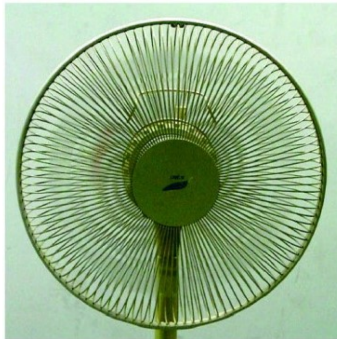
Figure 1. Example of moiré phenomenon. Moiré fringe pattern obtained by superposing front side grating and back side grating of wind fan
