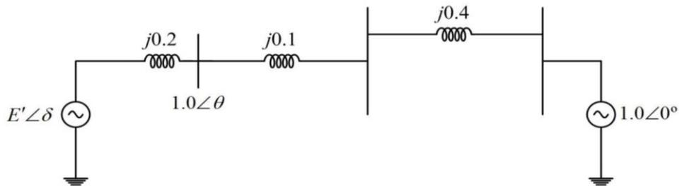
Figure 2. Simple power system after loss of a line.
