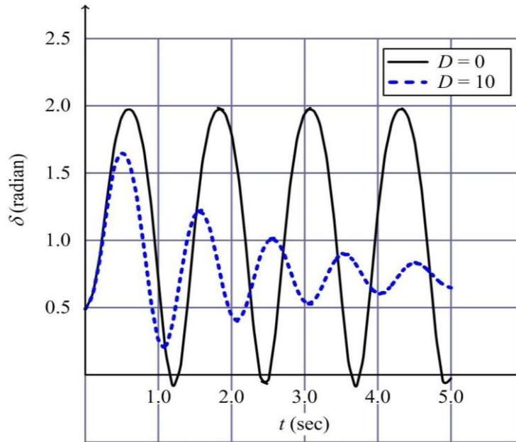
Figure 3. Rotor angle  $\delta$  vs time -  $D=0$  and  $D=10$ .
