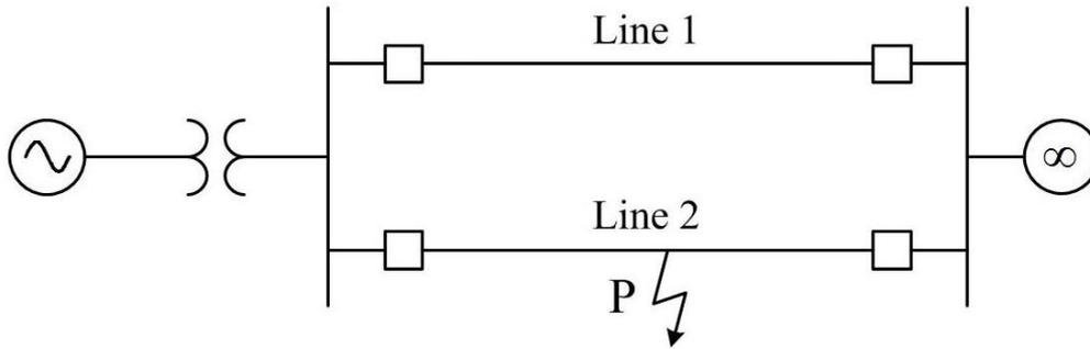
Figure 4. One-line diagram of a synchronous generator connected to an infinite bus.
