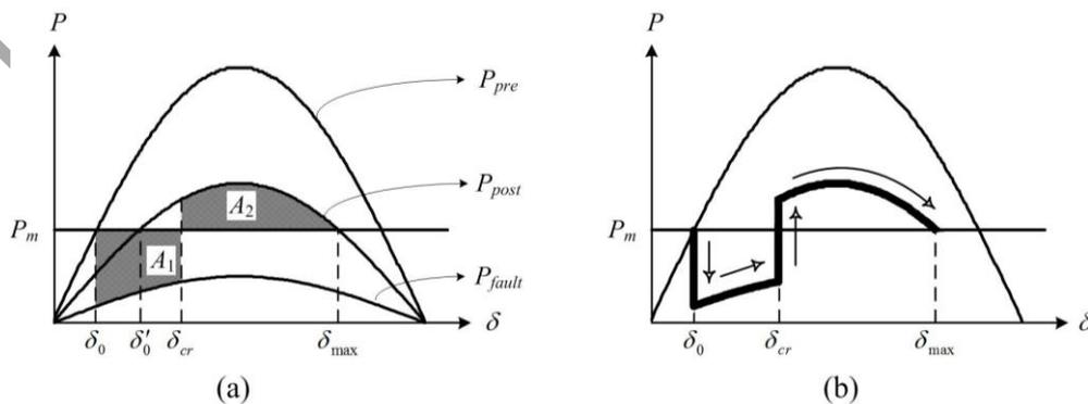
Figure 5. Equal area criterion. (a) areas  $A_1$  and  $A_2$ , (b) evolution of the machine angle.
