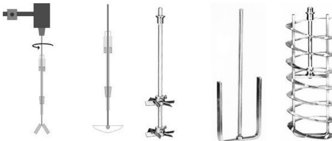
Figure 5. Several useful types of mechanical stirrer
