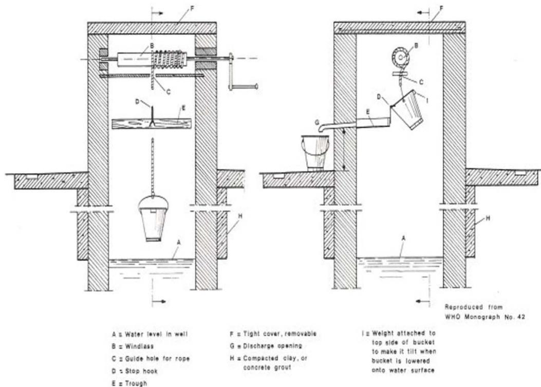
Figure 3. Sanitary rope and bucket system
