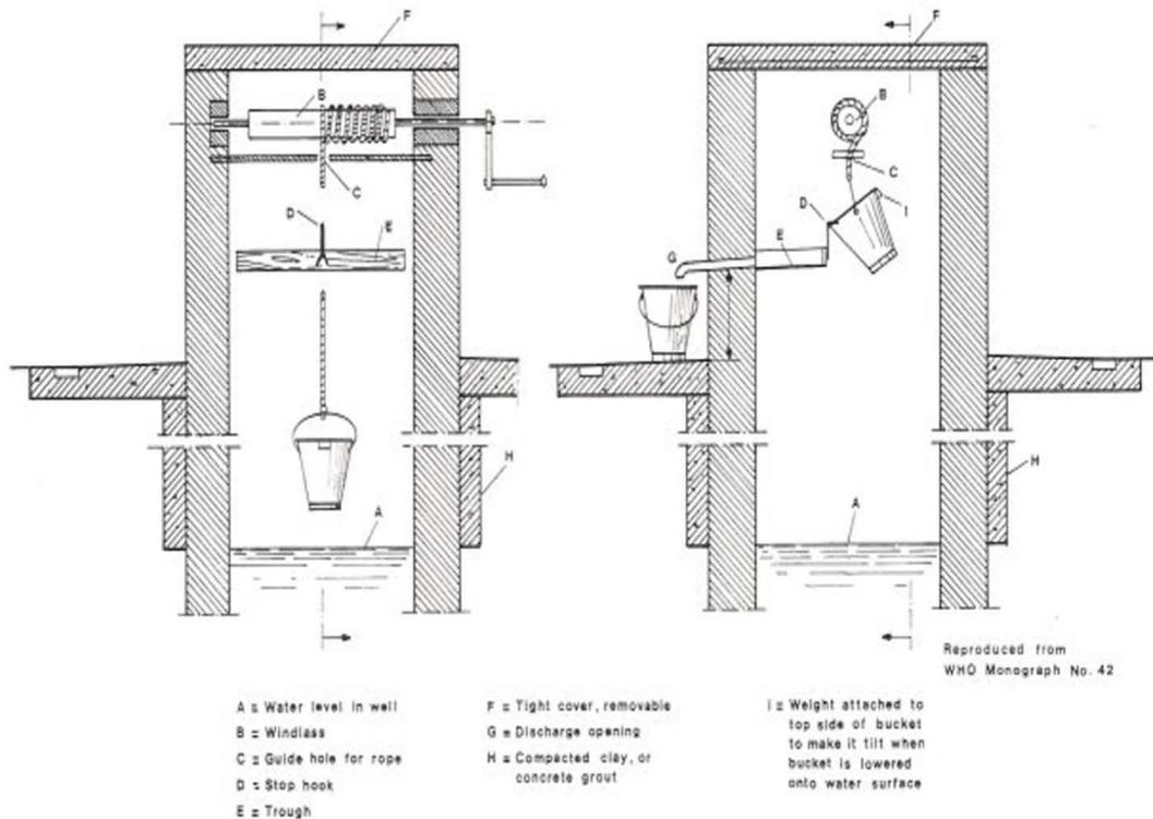
Figure 3. Sanitary rope and bucket system
