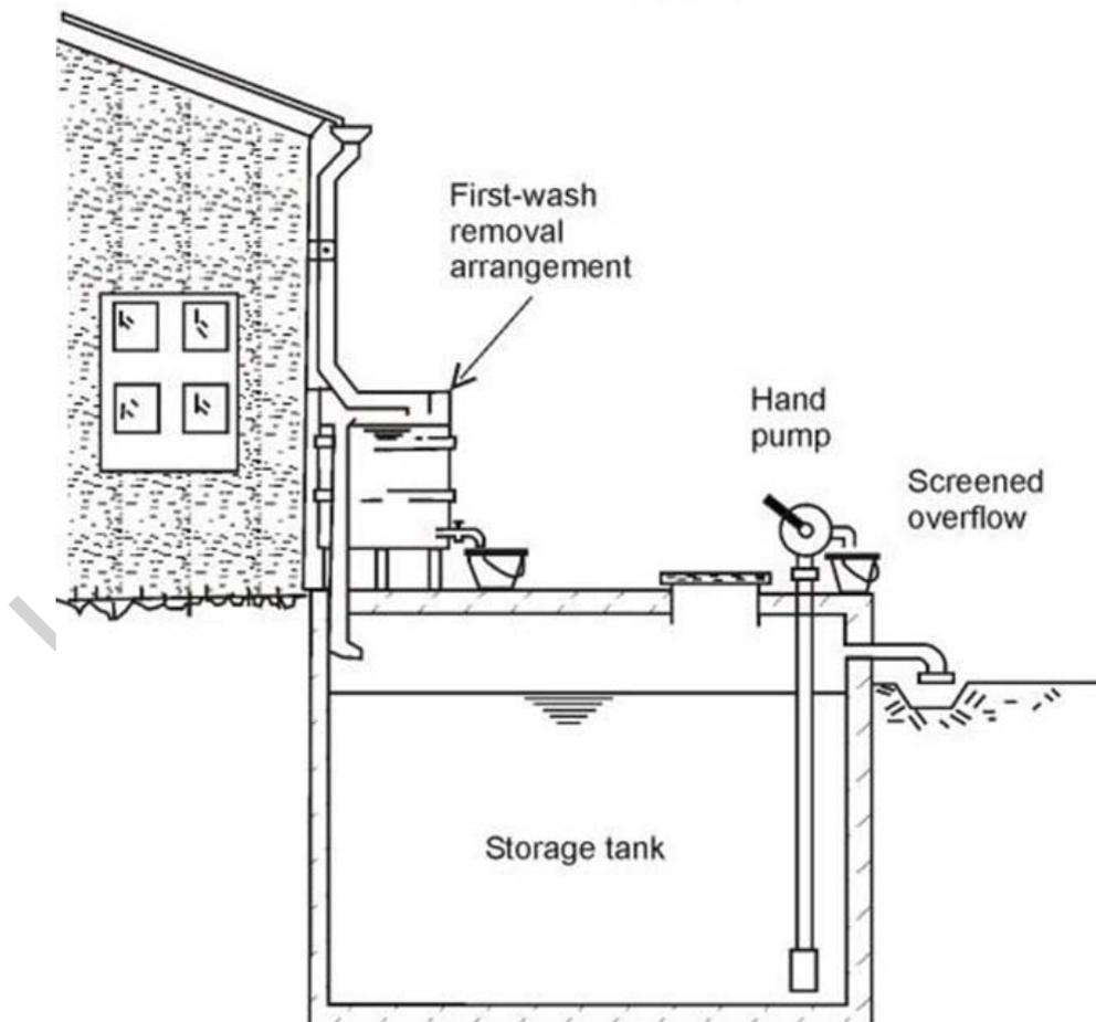
Figure 1. Roof catchment and storage
