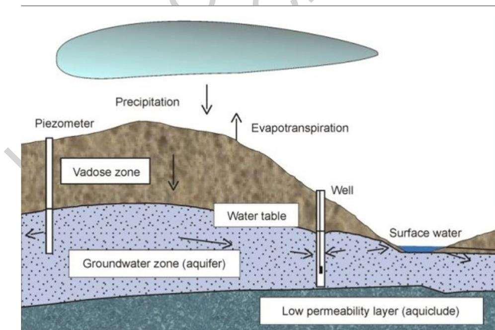
Figure 1. Schematic aquifer system
