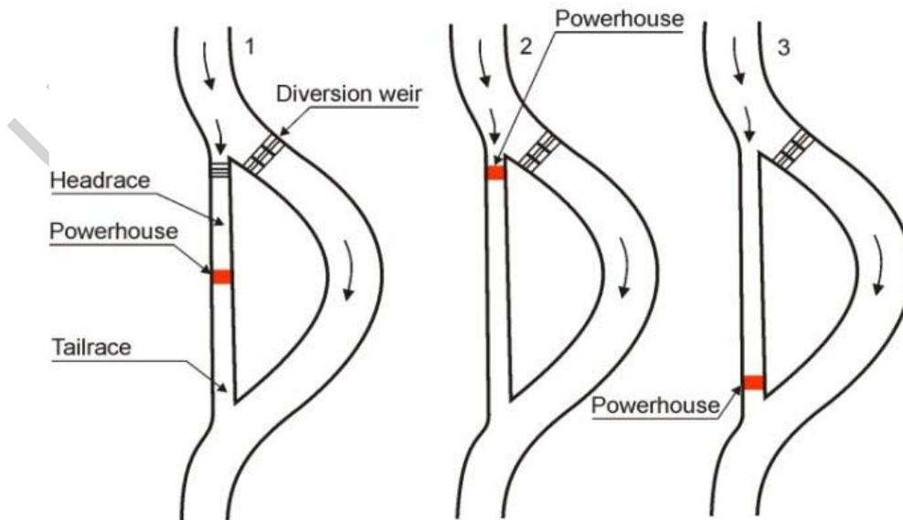
Figure 2. Location of the power station in the diversion canal
