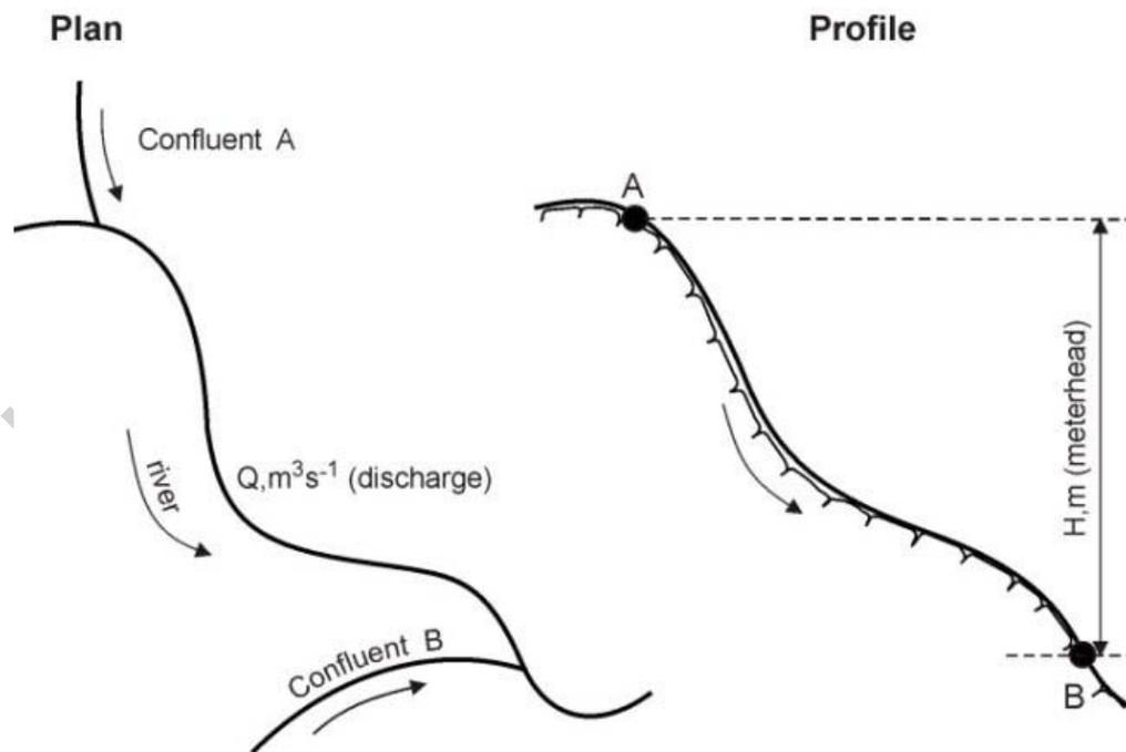
Figure 4. The river is divided into sections for calculating the power potential.
