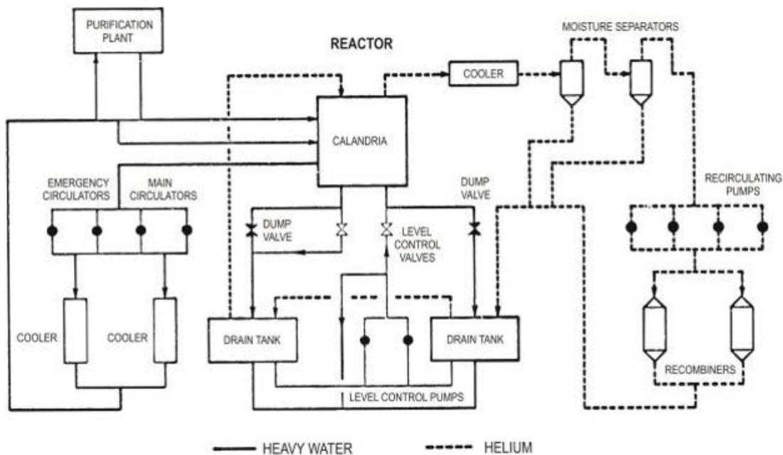
Figure 3. Heavy water moderator circuit
