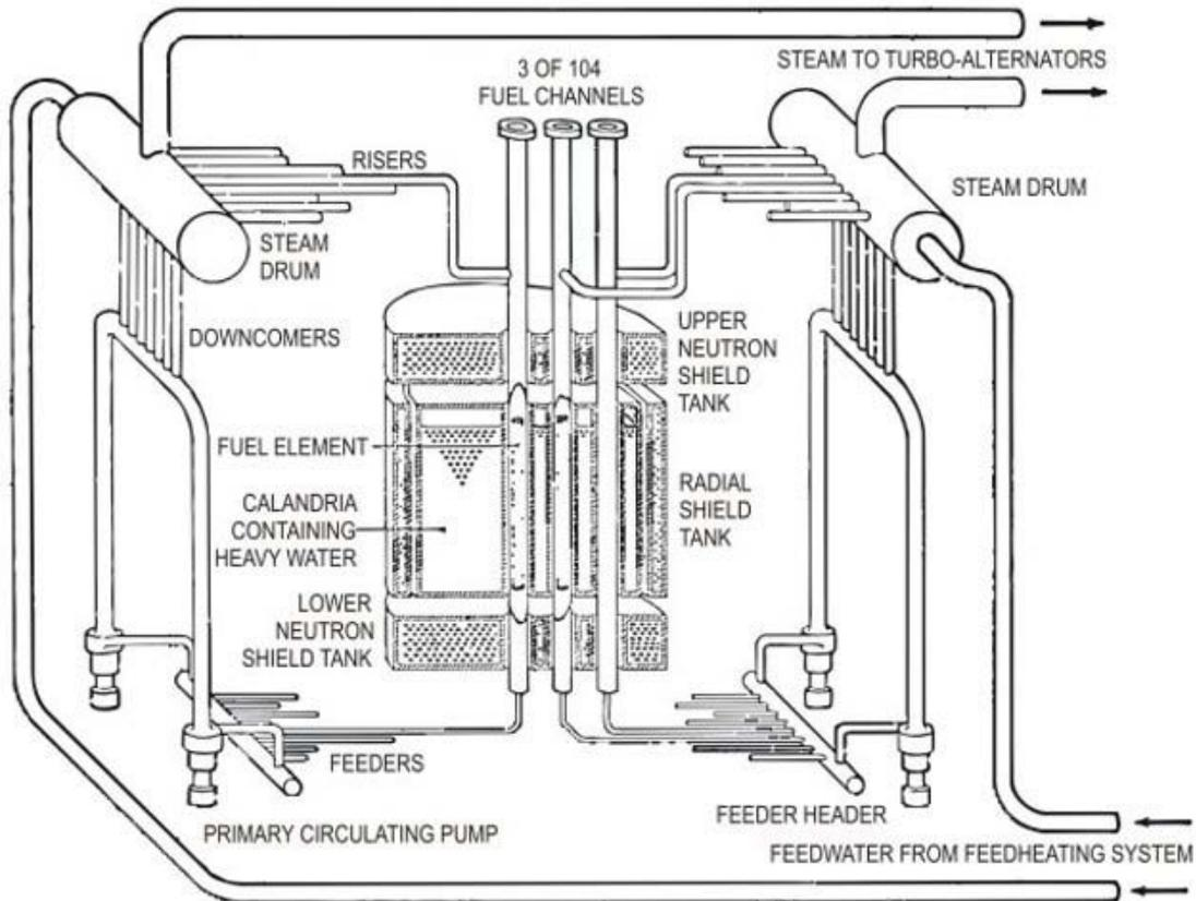
Figure 2. Reactor general arrangement
