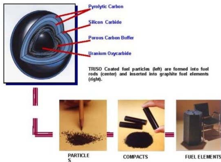
Figure 3: GT-MHR TRISO coated particle fuel
