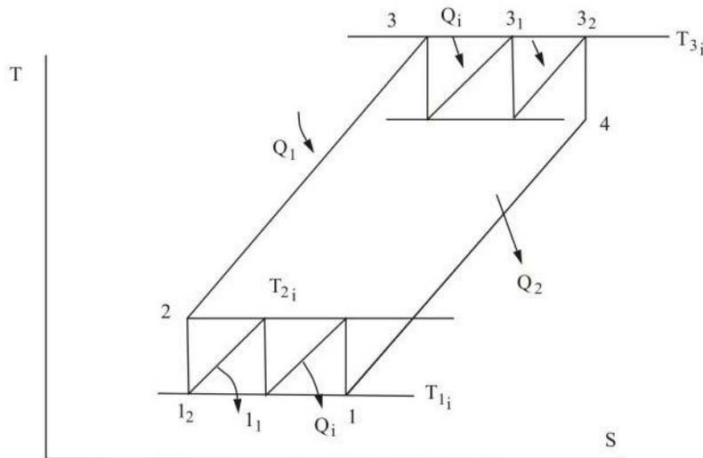
Figure 7 Ideal cycle with two intermediate coolers and two intermediate heaters
