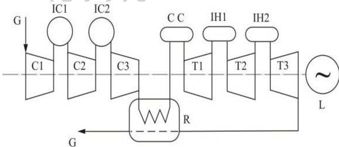
Figure 3. Scheme of GTU with intermediate cooling and intermediate heating
