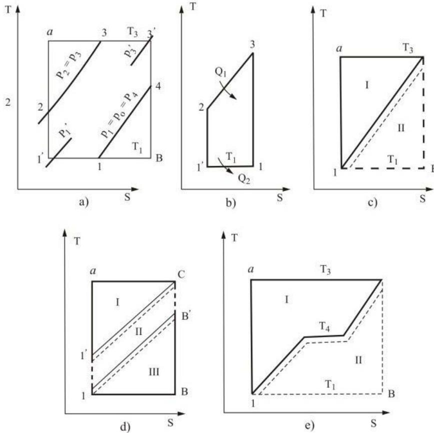
Figure 8 Ideal Carnot cycle (a), ideal Uvarov cycle (b)
