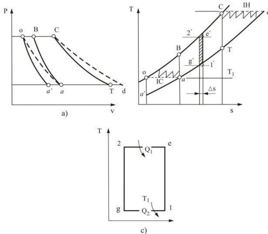
Figure 5 Ideal cycle with isothermal compression and expansion processes
