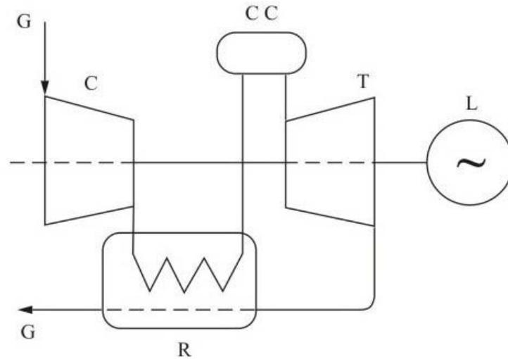
Figure 2. Scheme of the simplest regenerative GTU
