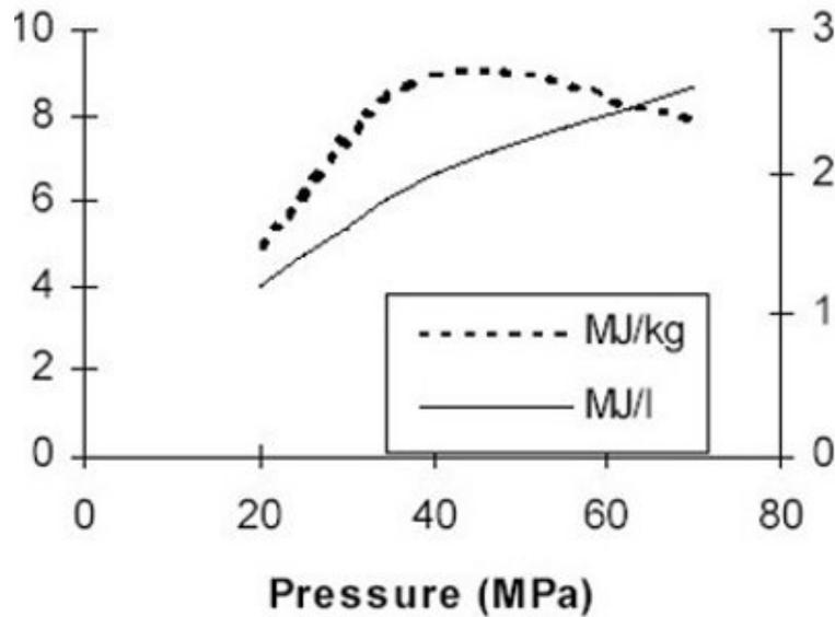
Figure 1: Energy density for gaseous hydrogen in cylinders
