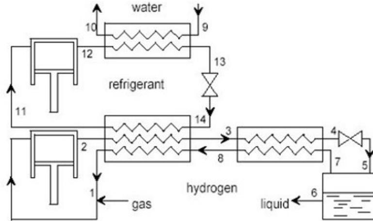
Figure 3: Schematic of a Linde plant for hydrogen liquefaction
