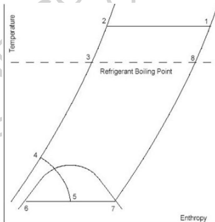
Figure 2: Linde cycle for hydrogen liquefaction.
