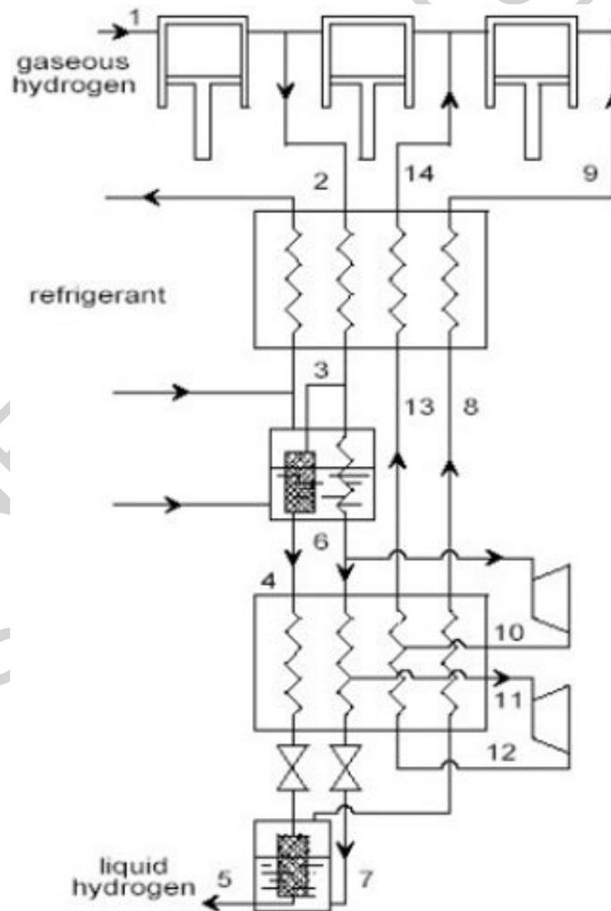
Figure 4: Schematic of a plant for hydrogen liquefaction
