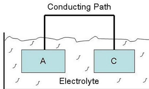
Figure 3. Laboratory Identification of the Four Corrosion Elements
