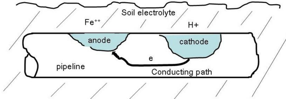
Figure 4. Corrosion Cell on a Buried Pipe
